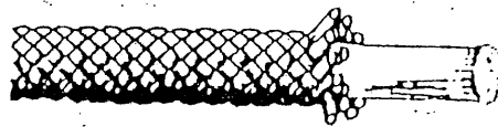
Fig. 2-14. Static kernmantle. A protective sheath woven tightly over a load-bearing parallel-fiber-bundle core.
